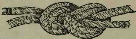
FIG. 24.—Double figure-eight knot (complete).
